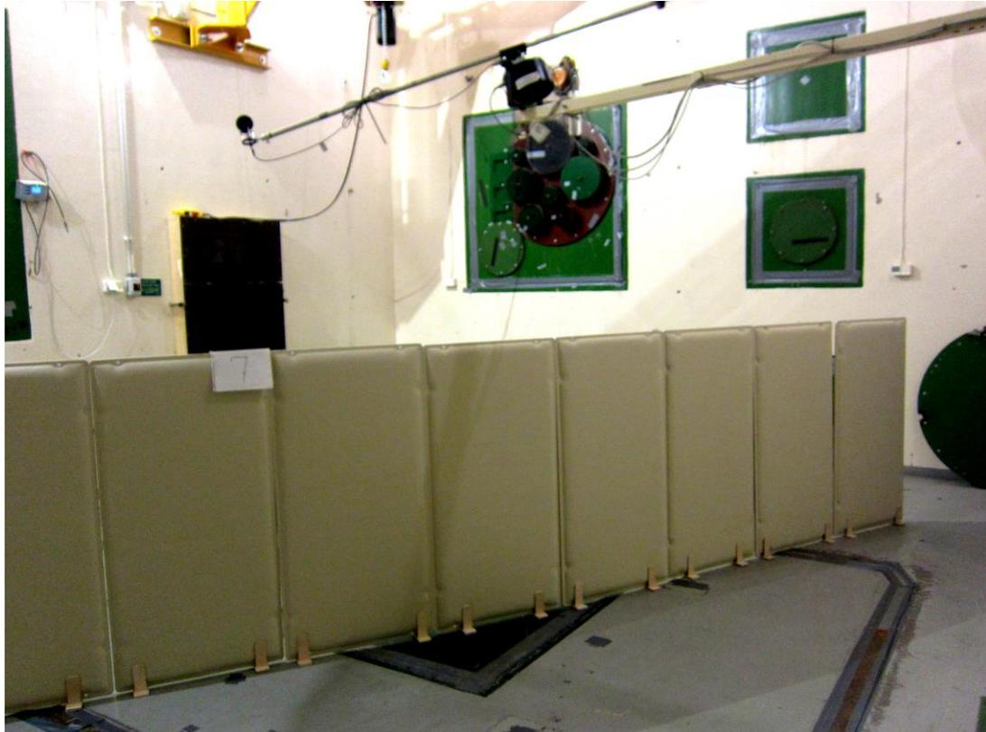
Determination of sound absorption and class of Yeseco Ilmava Acoustic Screen in a reverberation room according to SFS EN ISO 354-2003 and SFS EN ISO 11654-1997
